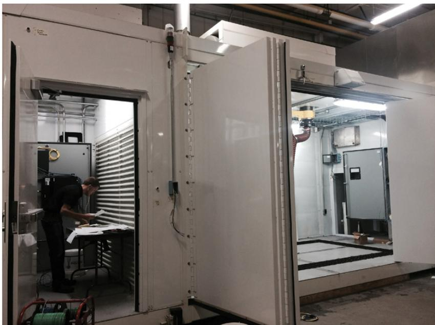
Along with the large climate cells, the CyberMetrix climate center includes a range of other testing systems, including natural gas and diesel dynamometers, cold and freezing chambers, altitude benches, thermal chambers, industrial ovens, SCR doser test stands and fuel contamination rigs.
